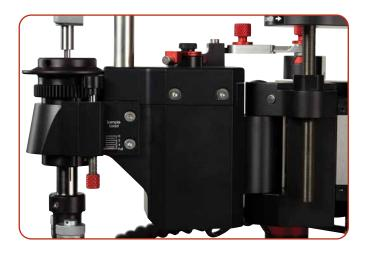
The gear-drive system allows preparation of larger, hard, tough or encapsulated materials. It delivers nonslip rotation for higher load-bearing applications.
