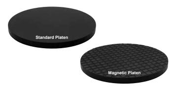
Precision platens are lapped parallel within 2  $\mu$ m and hard anodized for maximum wear resistance. They are used with plain or adhesive back discs. Magnetic platens combine a precision platen with a cross-hatched magnetic surface for maximum flatness and adherence. This allows all magnetic system cloths/abrasive discs or ferromagnetic discs to be utilized.
